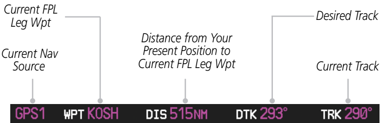
Figure 2-2 PFD Nav Status Bar Description
